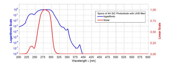
UVB+UVC SiC based UV photodiode A = 1.0 mm<sup>2</sup>
